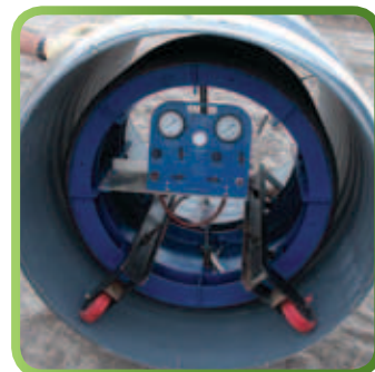
Joint Isolation Test
